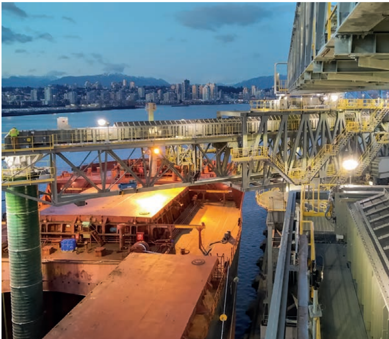
Triple ship loader for agri-food materials. P&H Fraser Grain Terminal, Vancouver Port (Canada)
