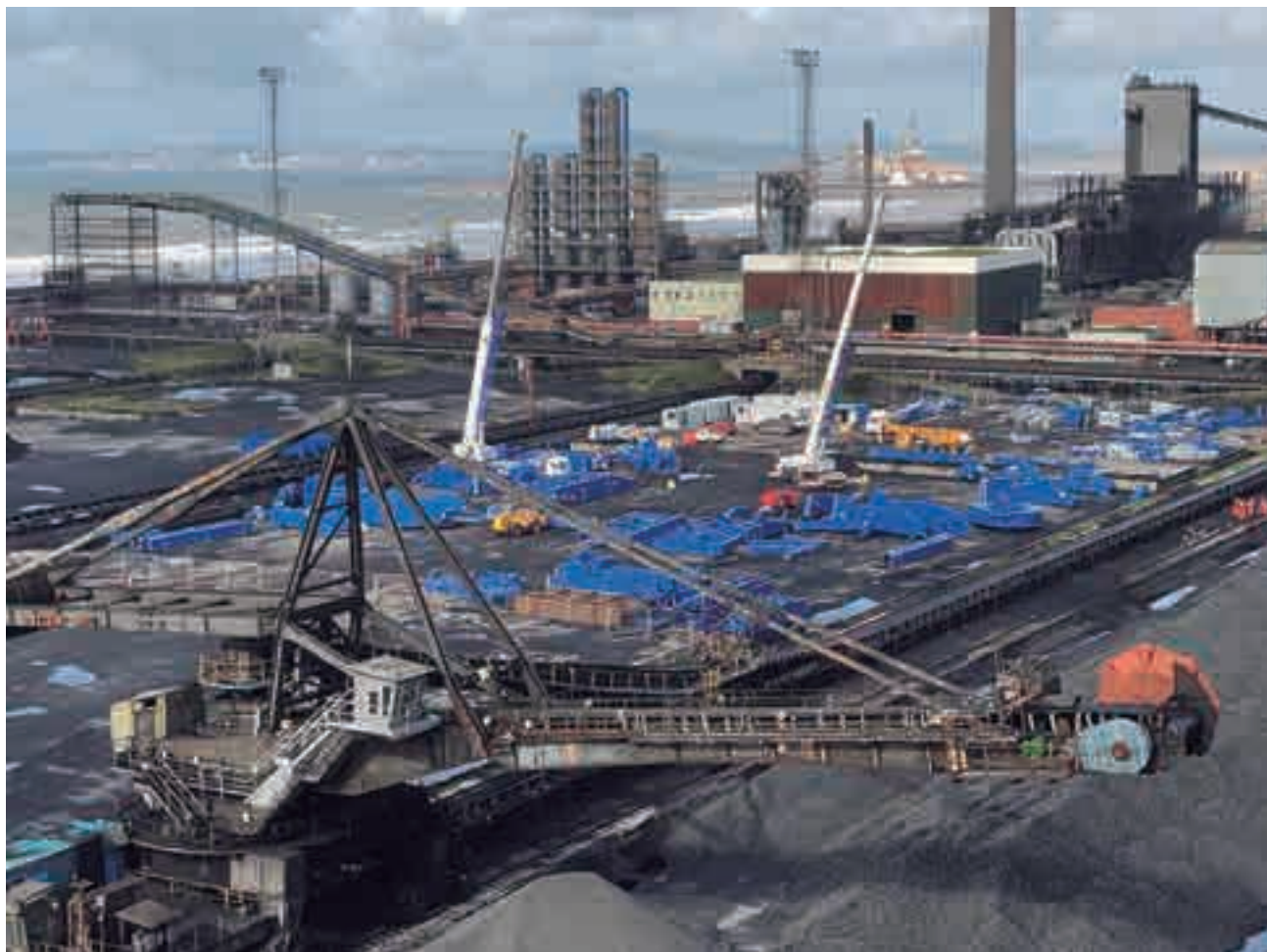
Bucket wheel stacker-reclaimer. Port Talbot Steel Making Plant. Wales, (UK)
