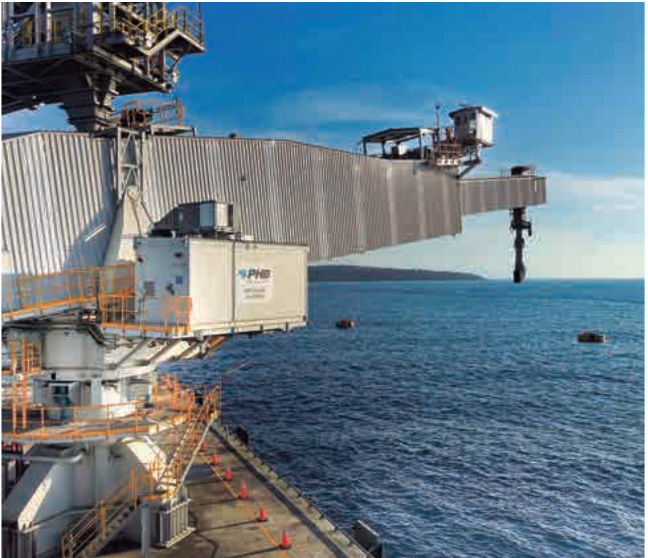
High capacity ship loader with telescoping boom. FIRST QUANTUM MINERAL. Punta Rincón ( Panama)
